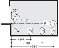
Bearing loads are transmitted to the pit floor by base plates of approximately 140 cm<sup>2</sup>, fixed by heavy duty anchor bolts to a depth of approximately 10–12cm. Base plate thickness min. 18 cm Concrete quality according to the static requirements of the building, but for the dowel fastening we require a concrete quality of min. C20/25. When fixing to waterproof concrete floors chemical anchors are employed (to be advised by WÖHR).
